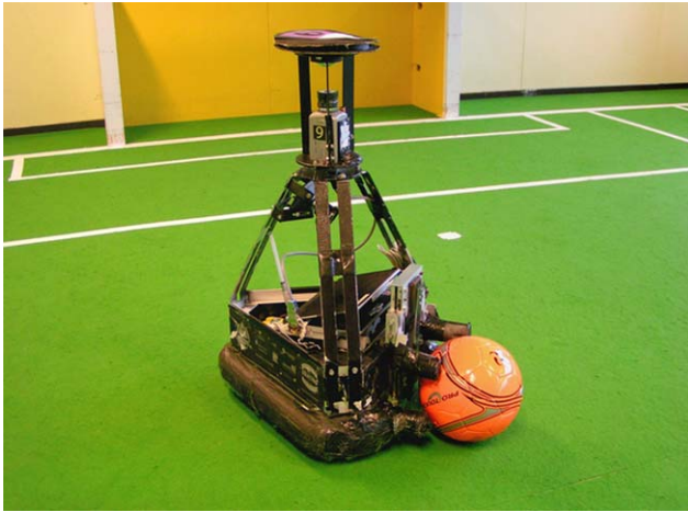
Fig. 13 Brainstormers MidSize league robot. The difficulty of dribbling lies in the fact that, according to the rules, at most one-third of the ball may be covered by the robot. Not losing the ball while turning, therefore requires a sophisticated control of the robot motion
