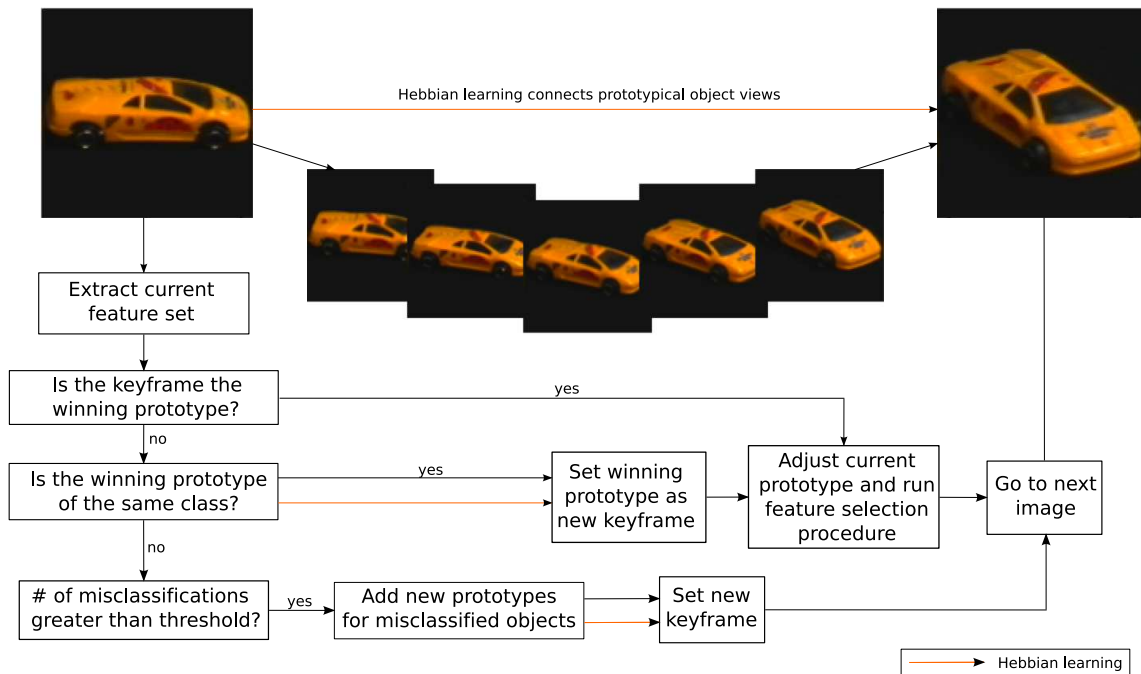
Fig. 3: A modular scheme of the framework showing the main learning process and handling of image sequences. At this level of description, it is still independent from a possible realization.
