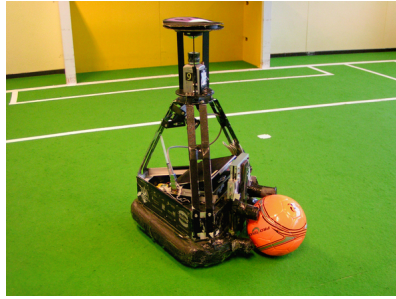
Fig. 6 Brainstormers MidSize league robot. The difficulty of dribbling lies in the fact, that by the rules at most one third of the ball might be covered by the robot. Not loosing the ball while turning therefore requires a sophisticated control of the robot motion.
