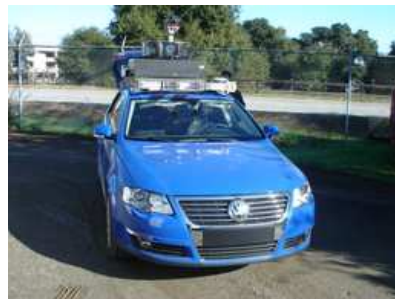
Figure 1. The car used is a VW Passat, equipped with additional sensors.
